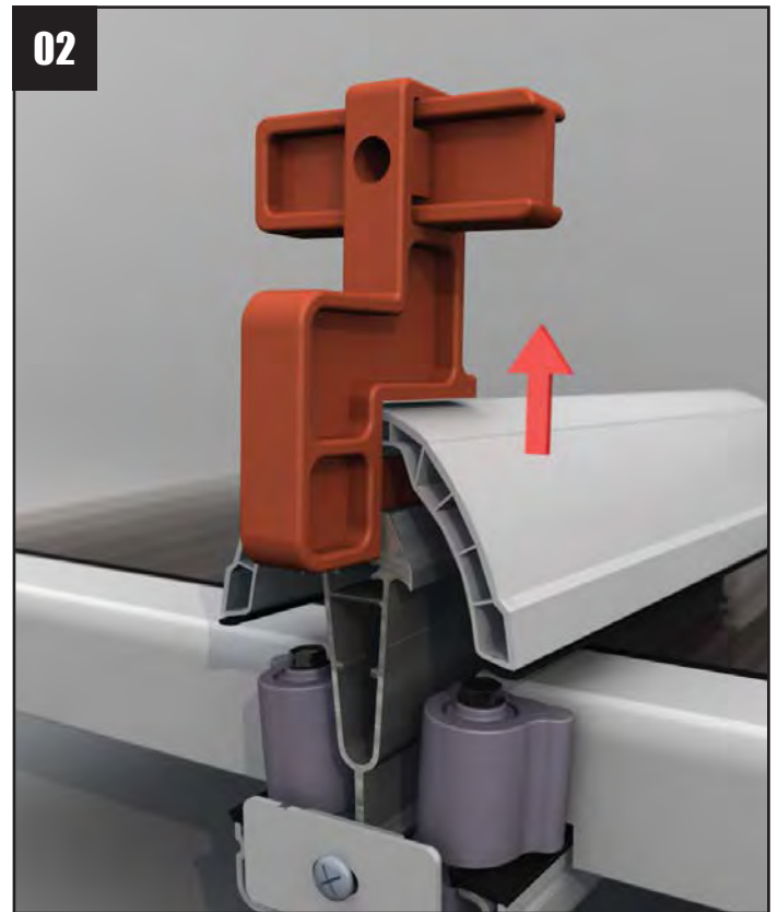
Lift the capping removal tool up, releasing the top cap legs from the aluminium.
