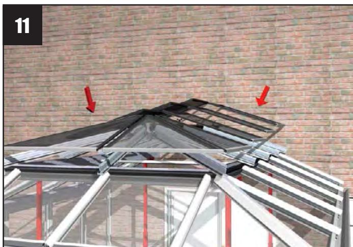
Glaze the upper pagoda roof, and complete all external works
