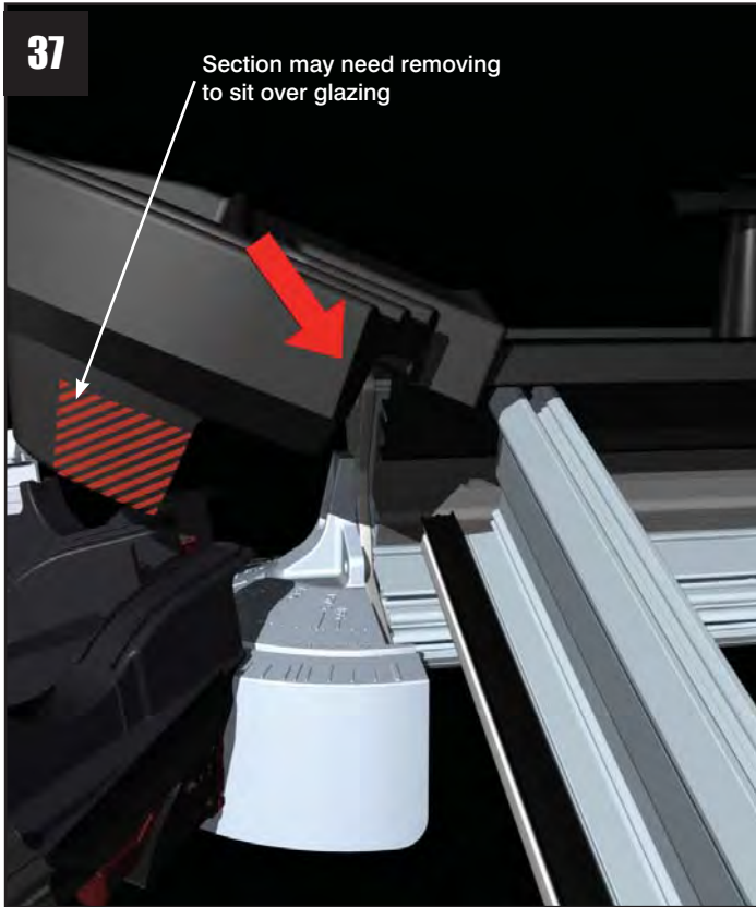
Take the 'soft touch' hub weathering shield and lift the flaps on the ridge rain baffle to insert. NOTE: If there are no side transoms in-line with the finial point, the weathering shield will need to be trimmed to suit to fit snugly over glazing.
