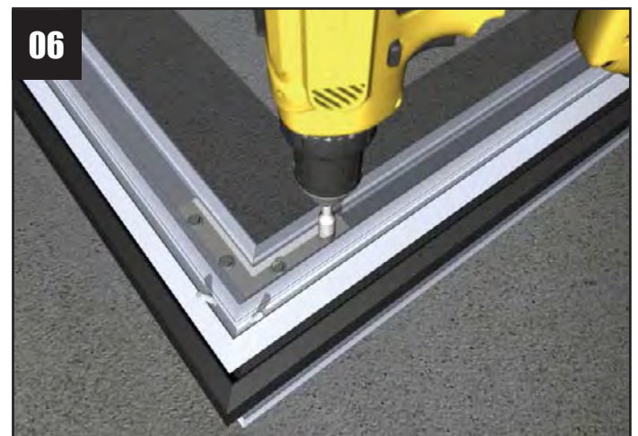
06 Fasten both fixings in both cleats on every corner.
