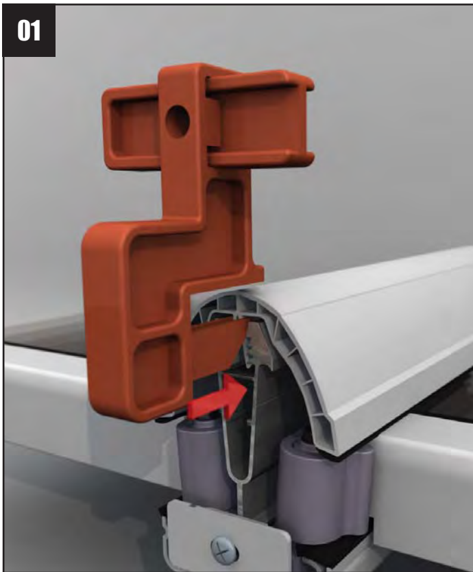
Insert the capping removal tool as shown.
