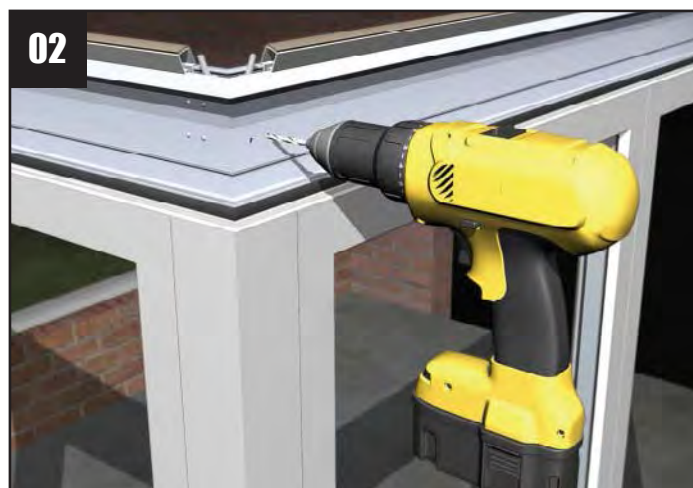
Two pilot holes already exist in the next piece of eaves beam – drill two more at 4.5mm diameter through the eaves beam and the cleat and then securely fit the four M5 x 12mm taptite screws.
