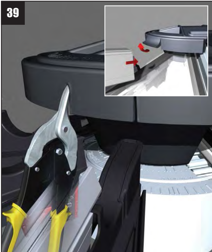
For the georgian hip bar, 'snip' two small cuts to facilitate the Georgian top cap sliding under - make sure the resulting flap is pulled forward.
