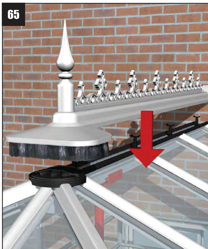
Offer up the complete ridge capping onto the roof. Please note. If a Ridgeflow ventilation unit is to be fitted, the air deflector must be attached to the PVCu top cap prior to its fitment. Refer to separate Ridgeflow installation guide.
