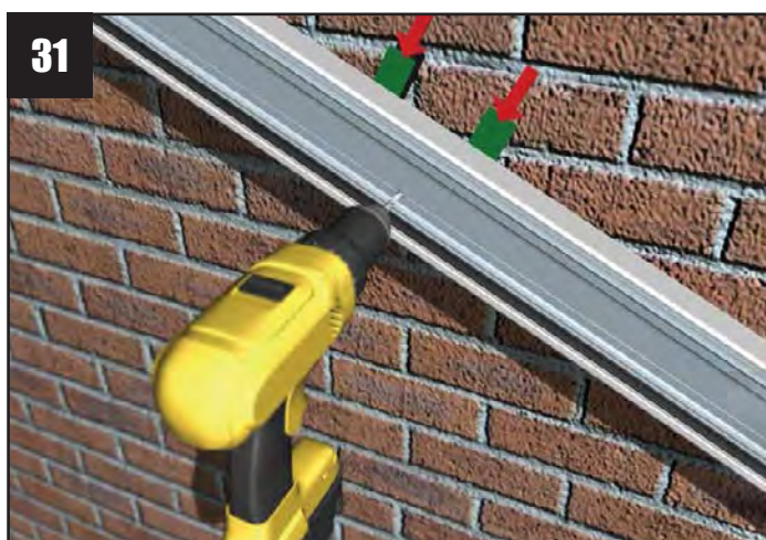
Drill the starter bars/masonry within 200mm of the ridge and eaves beam plus at least one more equidistant between the two. Pack out to support the starter bar behind each fixing before fitting the correct masonry anchor. If necessary pack behind the ridge too with aluminium shims.
