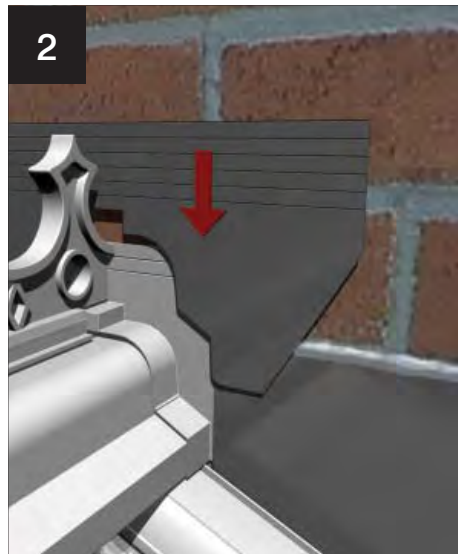
2 'Butter' with silicone and fit pre-cut saddle trim.
